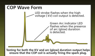
Simply press the 7" long antenna probe against the ignition coil and use the thumb-wheel to adjust the sensitivity until the LEDs begin flashing. Each time the unit detects a spark firing it will flash the bright LED strobe indicating sufficient kV and flash the green LED indicating sufficient Arc Duration. This allows the technician to determine if the coil is firing the spark plug consistently, intermittently misfiring or not firing at all.
